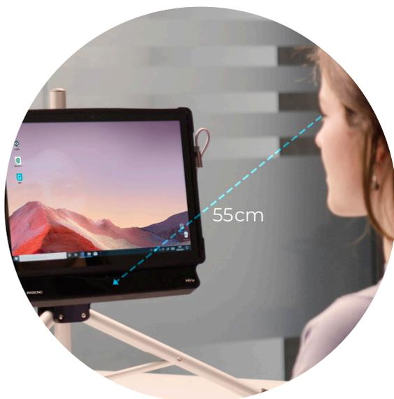
*If you want to use the eye tracker with larger screens, you can do so by changing the position of the camera and placing it further away from the screen.*
